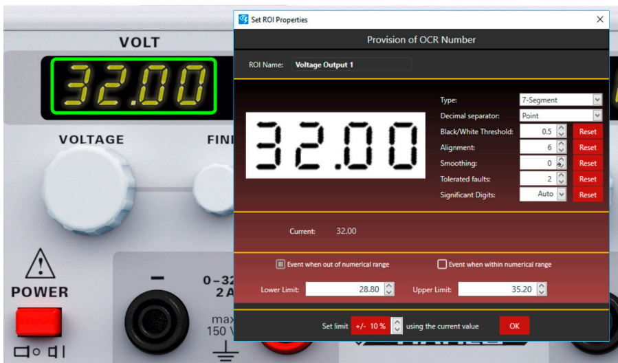
Checking a numerical test result with "OCR Number"
