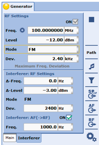
Frequency modulation with an integrated interfering signal.
